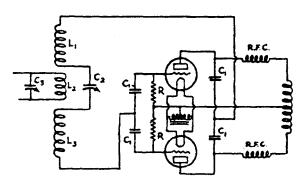
fig. 2. The nu8EX transmitter used for the first two-way 10-meter contact had a pair of 210 tubes in a self-rectified oscillator circuit. Alternating current at line frequency was applied to the plates of the tubes from the transformer at the right of the circuit (secondary only shown). With the low-C tank circuit and ac plate supply, the transmitter note must have been terrible! But it was good enough to do the job. (Drawing reproduced from the August, 1928, issue of QS7).
